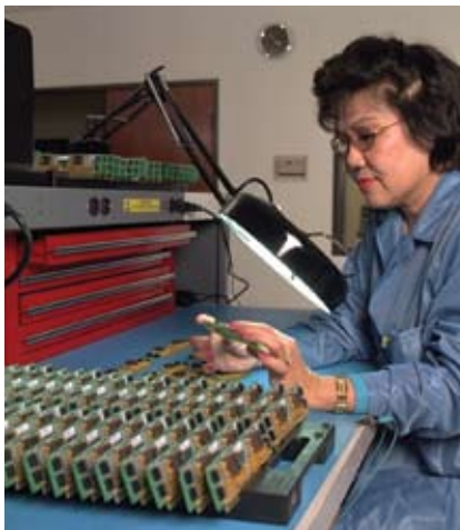
At Heads Up Technologies' facility, this electronics assembly technician performs a board inspection.
